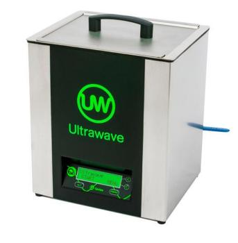
The **Qi-200** is a 12Litre ultrasonic cleaner with a menu driven, LCD control panel. This allows simple adjustment of cycle time (0 to 99mins or infinity mode), temperature (ambient to 80°C), ultrasonic power and frequency mode for precise and accurate processing.
