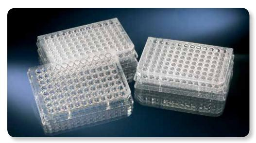
Round Bottom (U) 96-well Polystyrene Plates are optimized for robotics, automated readers and liquid handling systems.
