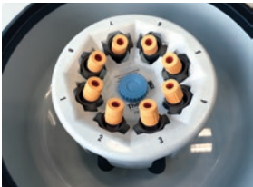
DualSpin rotor with swinging buckets
