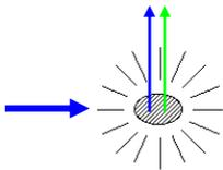
**2. Light from the laser(s) excites cell-bound fluorophores and is scattered by the cells.**
