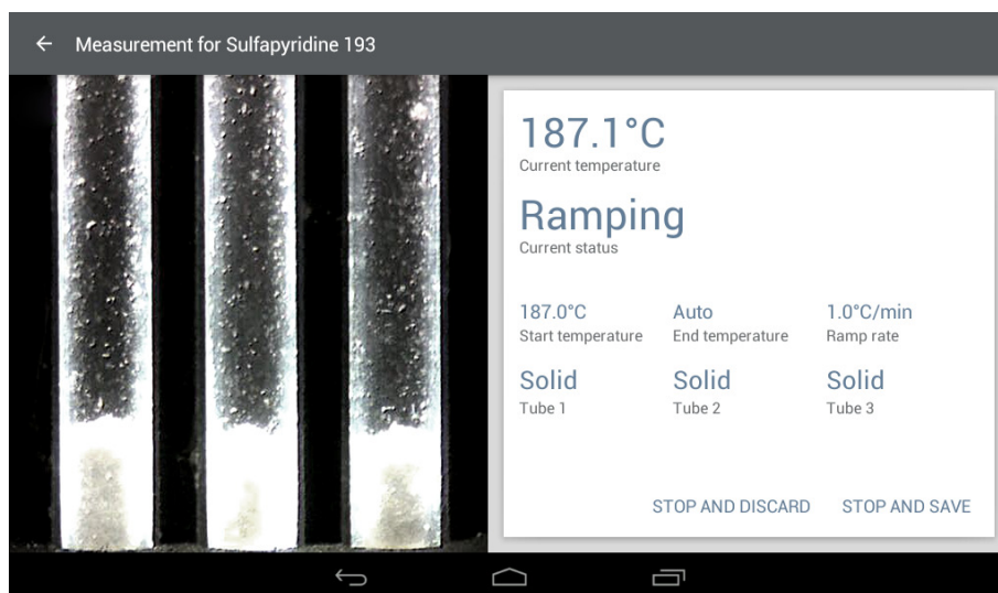
Run screen status 'Ramping'
