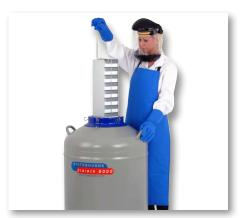
Quick,easy storage and withdrawal of racks, combined with exceptional holding times make the Biorack Series a leading choice
