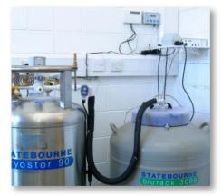
Biorack Autofill and Cryostor option (see next page) connected to Data logger low level alarm and autodialler.
