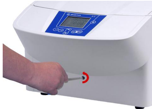
Fig. 11: Manual release of the lid lock
