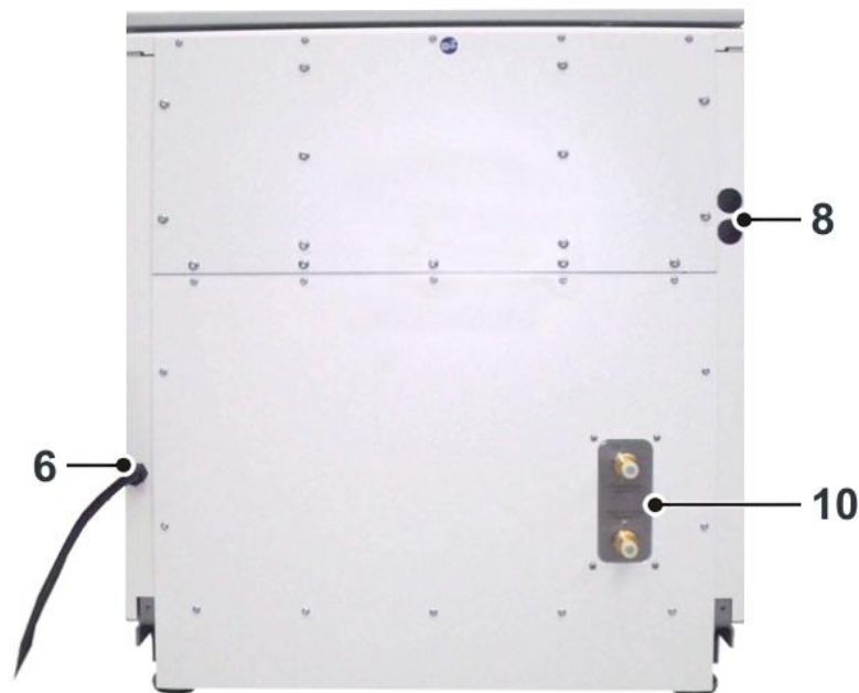
Fig. 4: Rear view of a water cooled centrifuge 1
