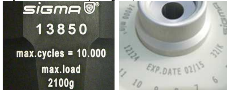
Fig. 5.9: Different service life – engraving on the bucket/rotor
