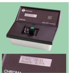
MODEL 252 (Non-programmable) The market leading analogue colorimeter has been brought into the digital age. The old familiar mirror parallax reducing combined Absorbance and %Transmission scale has been replaced by an LCD screen. It may still be used in education to establish the relationship between Absorbance and %T as both are displayed simultaneously.
