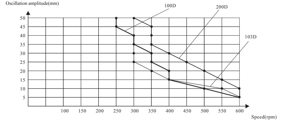
2.The adjustment of oscillation amplitude of ZHWY-103B multi-amplitude orbital constant temperature shaking incubator.
