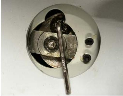
16.1.5. Keep M6 Allen key on the hex bolt to hold the shaking base as stationary, in the meantime, loosen the 10mm hexagon nut (4) with turning anti-clockwise with the socket spanner
