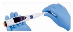
1. Unscrew the tip ejector collar counter clockwise and remove it.
