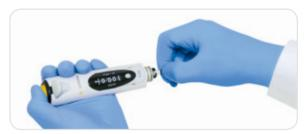
3. Unscrew the piston counter clockwise from the pipette.
