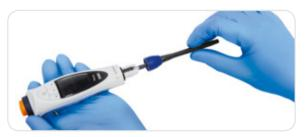
2. Unscrew the tip cone holder counter clockwise and carefully remove the tip cone holder, tip cone and spring.Remove the Safe-Cone Filter if fitted.
