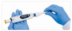
1. Unscrew the tip ejector collar counter clockwise and remove it.
