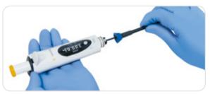
2. Unscrew the tip cone holder counter clockwise and carefully remove it along with the tip cone. Remove the Safe-Cone Filter if fitted.
