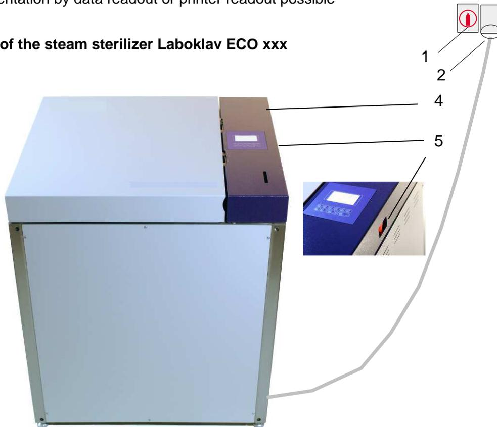
The Laboklav ECO should be operated while the normal laboratory working hours. If the device is not in use it should be switched off by the main power plug (5). Over night and on the weekends the central power plug (1) should be switched off. If that central power plug is missing please use the main breaker below the housing on the right side of the unit (4).
