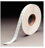
for sterilisation facilities to ensure that products have been exposed to the sterilisation process. Labels turn from blue to pink after exposure to 121°C for 3-10 mins, or 134°C for 0.5—2 mins.
