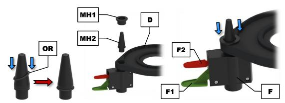
Fig. 7: Assembly of the clamping lid
