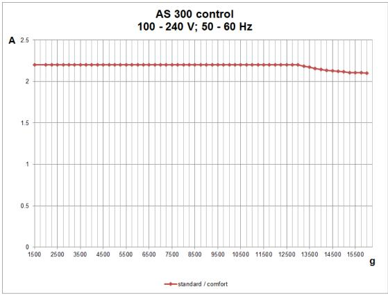
Fig. 12: Load diagram for the sieve clamping units "standard" and "comfort"
