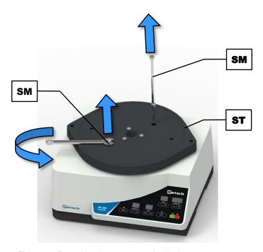
Fig. 2: Removing the transportation lock
