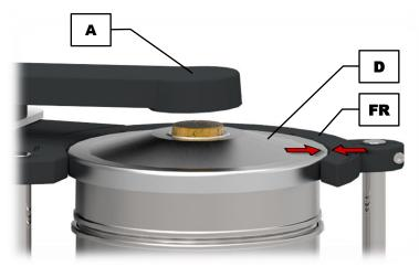
Fig. 9: Insert the sieve stack
