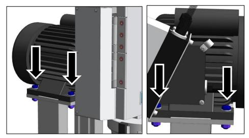
Fig. 12: Assembling the SM 100
