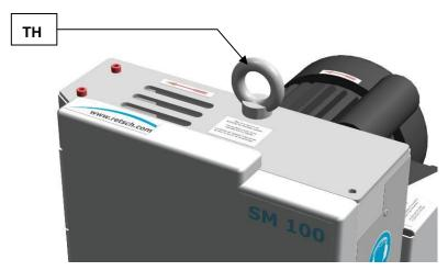
Fig. 2: Removing the transport aid
