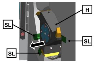
Fig. 28: Freely rotate the rotor
