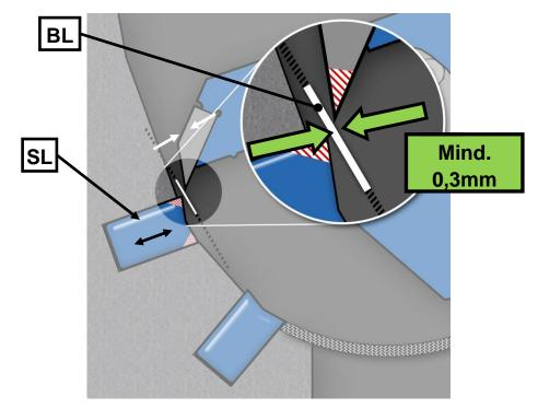
Fig. 29: Adjust the cutting gaps
