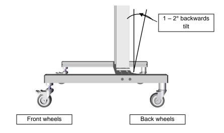
Fig. 17: Optimal alignment
