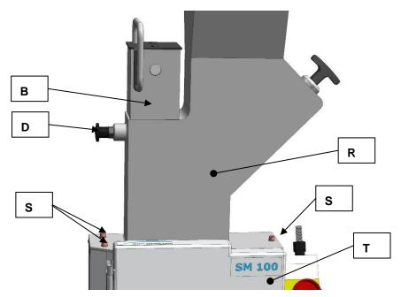
Fig. 14: Mounting the feed hopper
