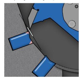
Fig. 26: Cutting gap
