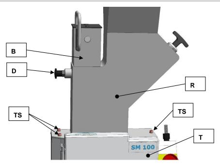
Fig. 37: Mounting the feed hopper
