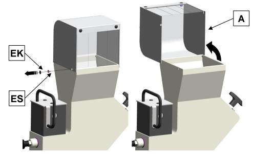
Fig. 36: Lifting up the feed hopper safety guard
