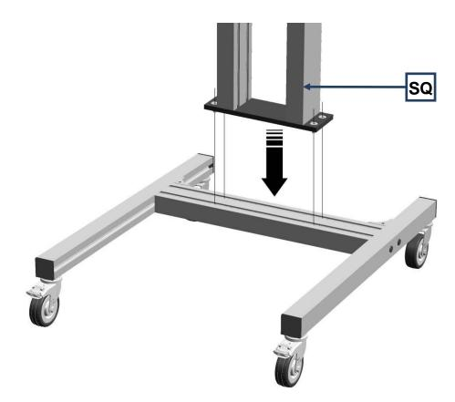
Fig. 9: Placing the crossbar on the stand
