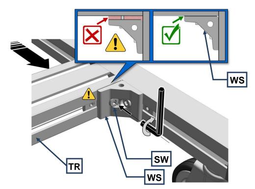
Fig. 5: Fastening the crossbar angle bracket
