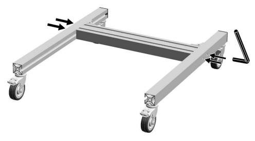
Fig. 6: Screwing the crossbar tight
