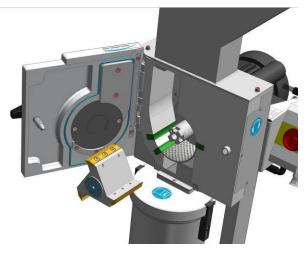
Fig. 38: Removing the rotor
