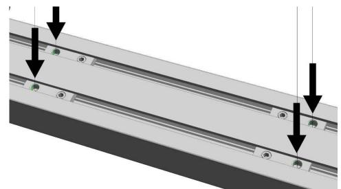
Fig. 10: Points for securing the stand
