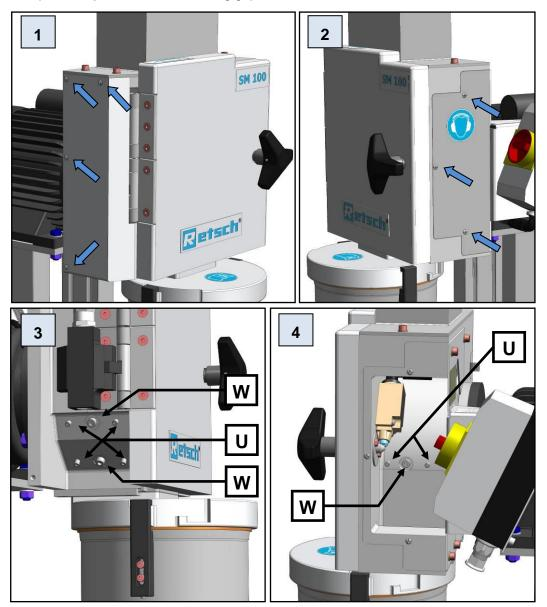
Fig. 27: Access to the cutting bars
