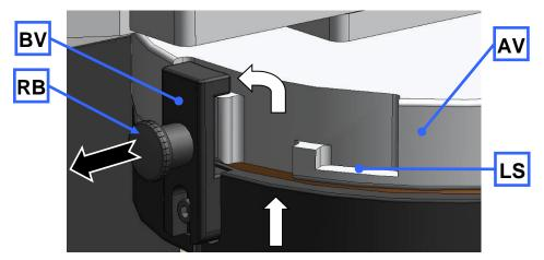
Fig. 23: Attaching and removing the filter unit
