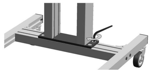
Fig. 11: Screwing the stand onto the crossbar
