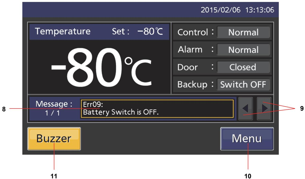
**8. Message display field:** The information of the operation monitor system, alarms or errors are displayed when fault occurs. Refer to page 45~47.
