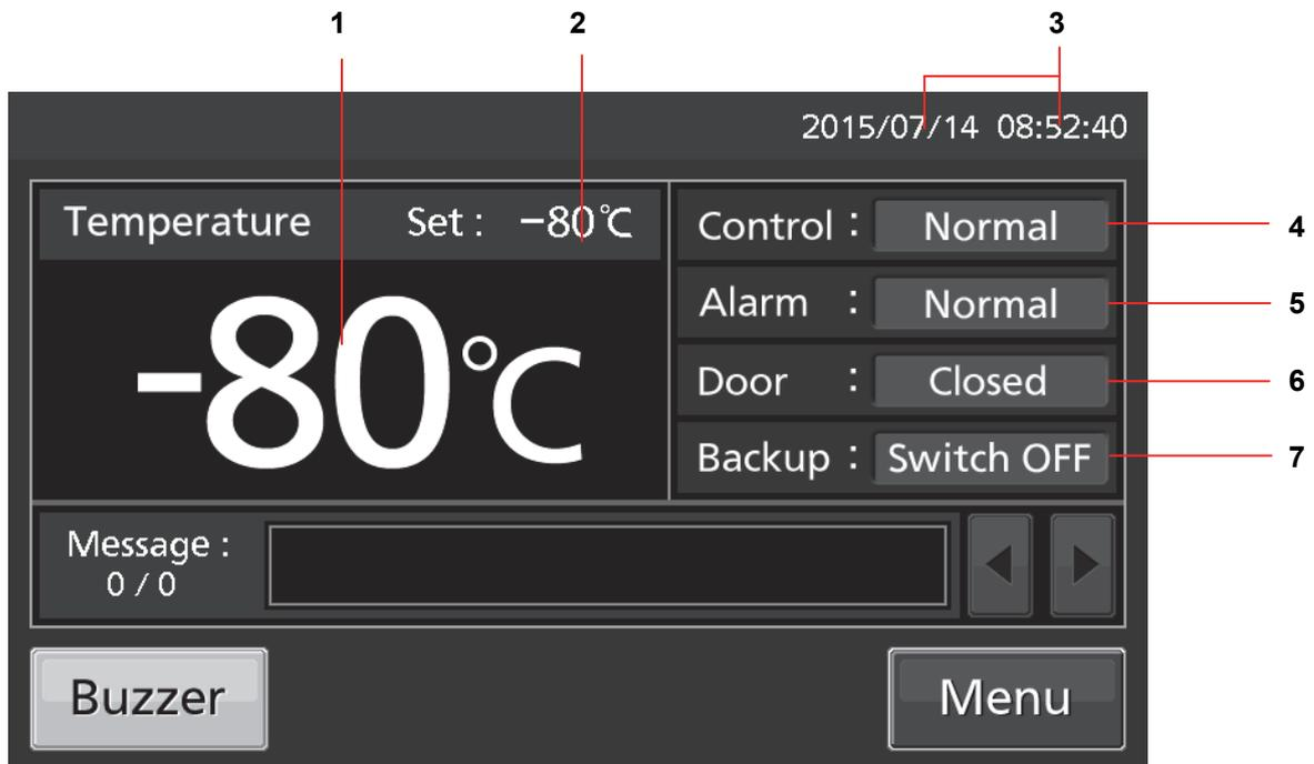
**1. Present temperature display field:** The current chamber temperature is displayed.
