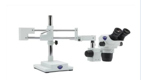
Binocular stereozoom microscope, 6.7x...45x, overhanging stand
