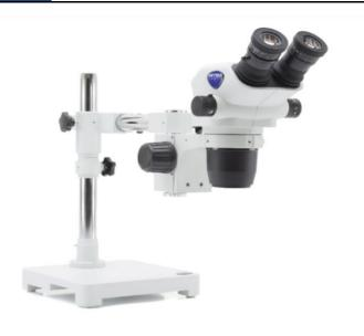
Binocular stereozoom microscope, 6.7x...45x, overhanging stand
