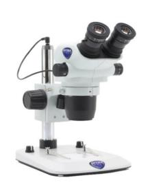
Binocular stereozoom microscope, 6.7x...45x, pillar stand, transmitted & incident light
