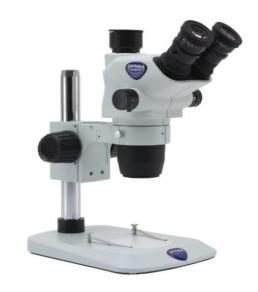
*Trinocular stereozoom microscope, 6.7x...45x, pillar stand*
