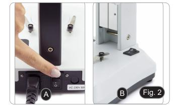
For SFX models, repeatedly press the touch button in order to change the light intensity.
