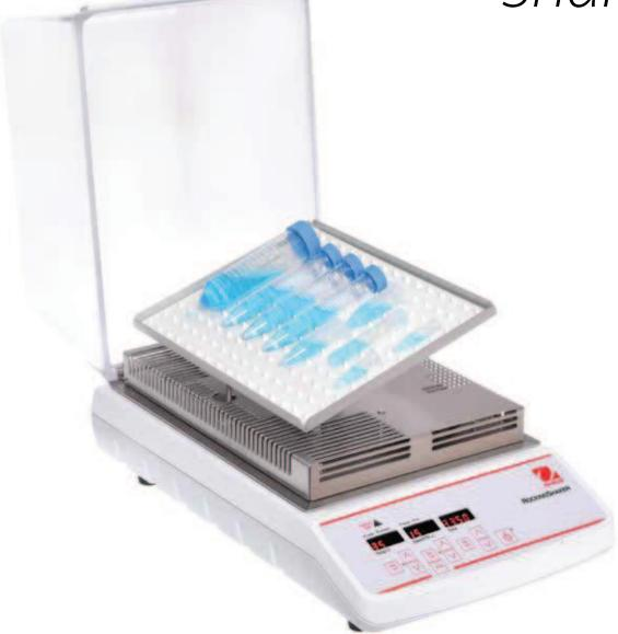
OHAUS Incubating Rocking and Waving Shakers are designed to incubate samples from 5°C above ambient to 65°C to provide accurate and repeatable results. Rocking shakers provide a see-saw like motion, while waving shakers offer a smooth, low-foaming three-dimensional "wave" motion. All models feature LED displays with touchpad controls. Both models include safety features that protect both the user and samples.
