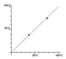
Verify the performance of the temperature control system digital display units undergo a factory calibration procedure which calculates the temperature values over the operating range of the equipment from 2 reference calibration points.
