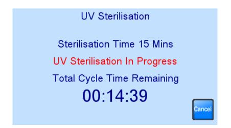
If the safety screen is removed or the button is pressed the cycle will terminate and the normal running screen will be displayed
