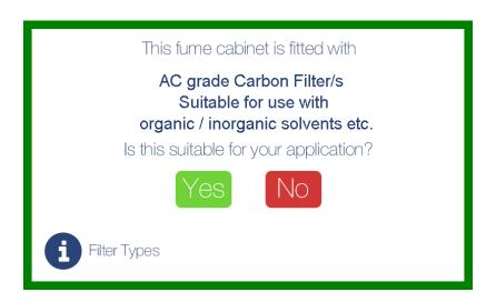
If the procedures carried out inside the cabinet are always the same this screen can be bypassed in the Supervisor Settings (see page11) When the filter type has been accepted the normal running screen below is displayed.
