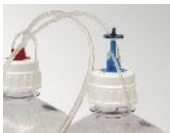
Biological filter on wash reagent bottle
