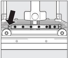
Place the track in the holder in the mobile unit and screw firmly in place.
