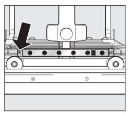
Unscrew the track with AWK (using an allen key) and remove from the retainer.
