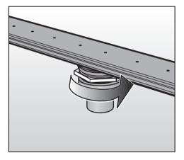
Use an SW 60 spanner to loosen the connection and then pull the spray arm upwards or downwards.
