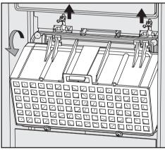
Remove the coarse filter housing.
