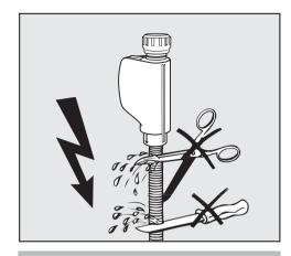
Do not cut the inlet hose or damaged in any way.
