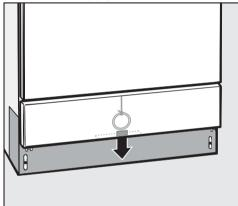
Remove the service panel and pull the ring of the emergency door release down.
