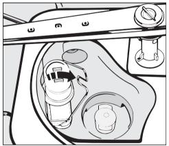
Lift up the non-return valve and rinse it under running water. The ball inside should move freely.
