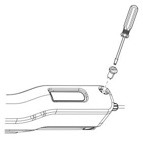
2 Screw the connector into the filling opening and tighten it.
