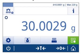
After a short period of time, the weighing pan is stable. The unstability symbol **O** disappears and the value in the weighing value field becomes **dark blue** again.
