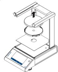
Remove weighing pan, pan support and bottom plate.
