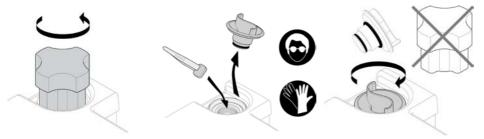
1-Using the tool, unscrew the 2-Remove the plug and insert 3-Screw the plug back: make sanitation port cap. the tablet in the port. sure the o-ring is in place.
