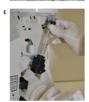
• Pull the UV Lamp out of the UV housing by its electrical cable (E).
