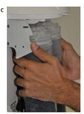
• Remove the SynergyPak cartridge(C).
