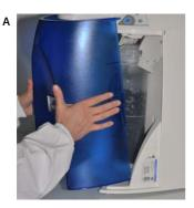
• Open the front cover to go into STANDBY mode (A).
