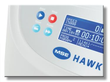
Maximum speed Maximum RCF Maximum Volume 18000 rpm 24270 xg 400 ml
