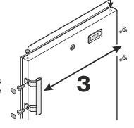
Transfer pin on hinge bracket to the opposite side.
