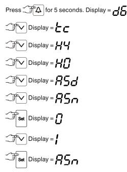
Automatic reactivation of the audible warning signal is now active.
