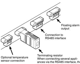
When connecting several appliances via the RS485 interface, the terminating resistor must remain on the last appliance. Remove the terminating resistors from the appliances in between.
