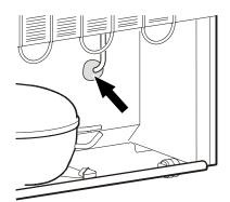
Important! Close the sensor cable opening at the back of the appliance with the sealant provided.
