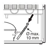
1. Drill marked section on the back of the appliance.
