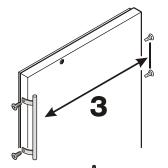
Transfer pin on hinge bracket to the opposite side.
