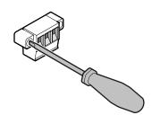
Remove the terminating resistors from the appliances in between.
