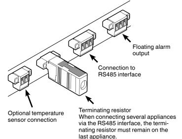
The connectors are secured with screws. To remove the connectors, undo the left and right screws.
