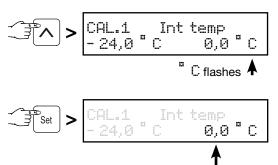
The temperature correction value flashes and can be changed using the buttons v or  $\lambda$ .
