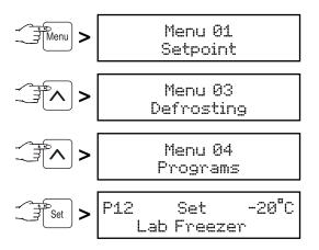
Press the set button to accept the new setting or the Menu button to cancel the procedure without saving.
