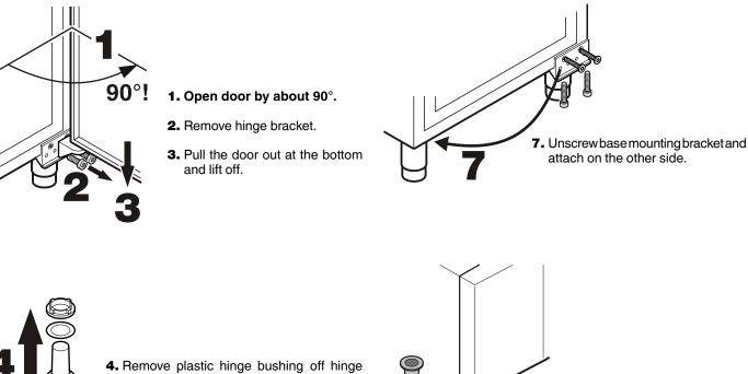
Remove plastic hinge bushing off hinge bracket.
