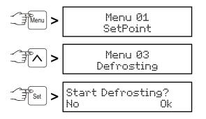
Press button  $\bigcirc$  to start defrosting or press the **Set** button to cancel the procedure.
