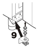
**9.** Insert hinge bracket in lower door mounting and screw to base mounting bracket.
