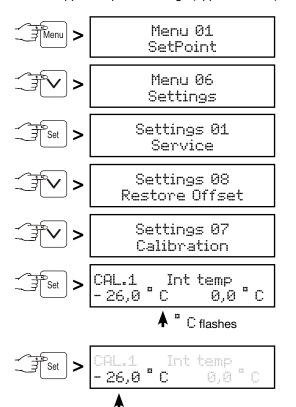
The temperature range display flashes and can be changed using the buttons  $\checkmark$  or  $\land$  (e.g. -1°C).
