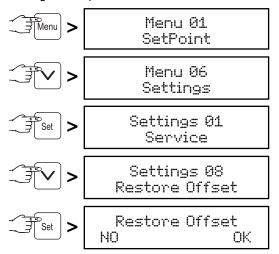
Press button  $\bigcup$  to set the temperature correction values for CAL1, CAL2 and CAL3, respectively, to 0 or cancel the procedure without any changes by pressing the st button.
