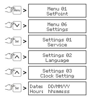
The value to be changed flashes and can be changed by pressing the buttons  $\checkmark$  and  $\land$ .
