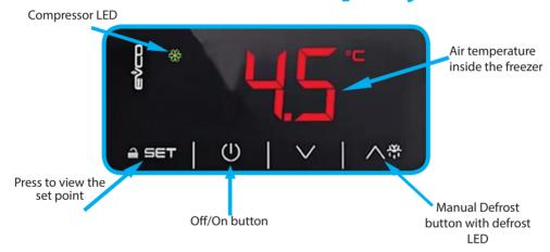
Your fridge is preset to  $5^{\circ}$ C so you do not have to program the set point. To check the set point, simply press the  $\triangle SET$  button.
