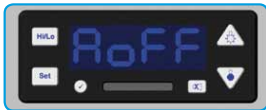
Figure 2 - Alarm mute display
