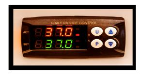
The programmed temperature, Set Point (**SET**) is displayed in **Green** and the Actual Chamber Temperature inside the Warming cabinet Inner Chamber (**ACT**) is displayed in **Red**
