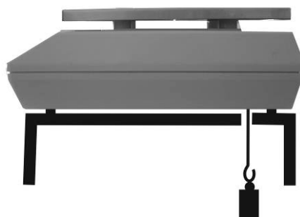
Fig. 1: Setup of balance for underfloor weighing
