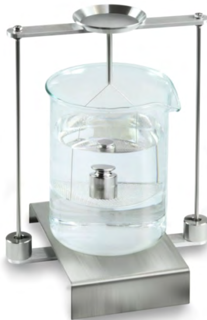
Fig. 2: Density determination set YDB-03 “weighing in test liquid“
