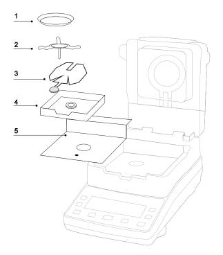
Open heating hood and remove all parts in the right order and clean. Please do not use aggressive cleaning agents (solvents or similar agents), but a cloth dampened with mild soap suds. Ensure that no liquid penetrates into the device. Polish with a dry soft cloth.
