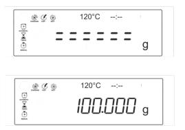
After successful adjustment the balance automatically returns to weighing mode, "100,000 g" will be displayed. Take away adjustment weight.
