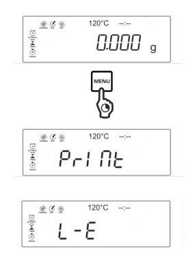
Acknowledge with LENTER. The protocol of the measurement carried out as last is displayed under the ident number "1". The instrument stores the last five protocols (ident number 1 -5). With every new measurement, the ident number One will be overwritten.
