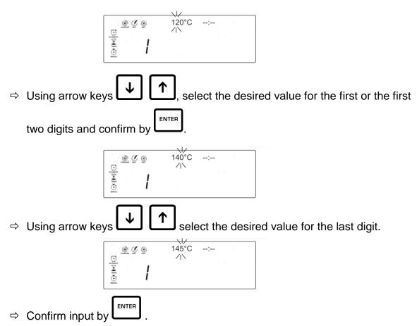
If as switch-off criterion **<AUTO>** or **<MANUAL>** is selected, the parameter setting is finished here. All parameter settings will be applied to a subsequent drying process and displayed on screen. All settings are stored under the ident number <1> until a new method is allocated to the ident number.
