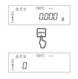
After pressing <sup>MENU</sup> the first ident number <0> will be displayed. This memory location is provided for the factory settings (standard drying 120°C, automatic switch-off) and cannot be changed.
