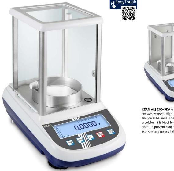
KERN ALJ 200-5DA with optional ioniser II, see accessories. High-precision semi-micro analytical balance. Thanks to its high level of precision, it is ideal for calibrating pipettes Note: To prevent evaporation we recommend economical capillary tubes (see standard 8655)
