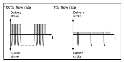
Fig. 4: Low-pulsation operating principle
