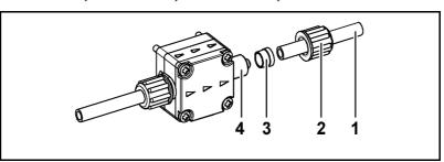
Fig. 12: 4/6 hose / clamp ring connection fitting (FEM)
