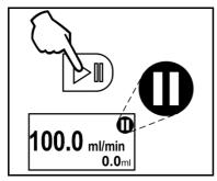
Fig. 20: Interrupting a pumping operation
