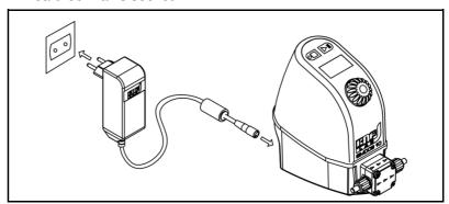
Fig. 11: Electrical connection
