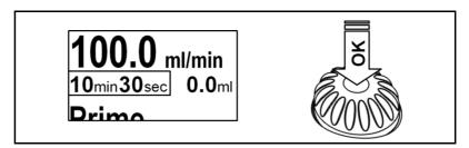
Fig. 25: Confirming the setting value by pressing the control knob
