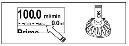
Fig. 23: Select the framed lines by pressing the control knob.
