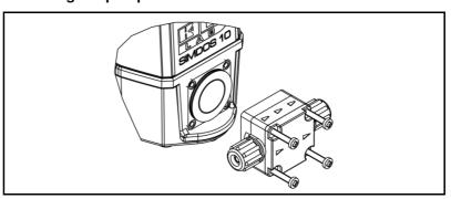
Fig. 56: Removing the pump head
