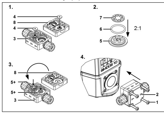
Fig. 59: Refitting the pump head
