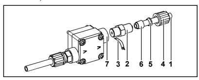
Fig. 13: 4/6 hose / cutting ring FT connection fitting
