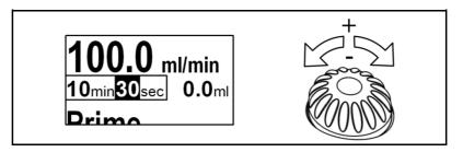
Fig. 24: Inverted display of editable values
