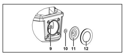
Fig. 58: Replacing the pump diaphragm
