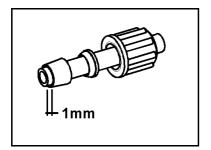
Fig. 14: Position of cutting ring and sealing ring on hose
