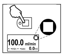
Fig. 21: Stopping the pumping operation
