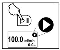
Fig. 19: Starting the pump
