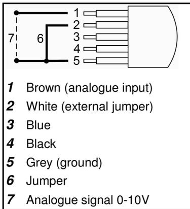
Fig. 17: RC cable jumper
