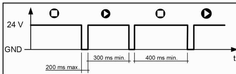
Fig. 21: Start/Stop pulse actuation
