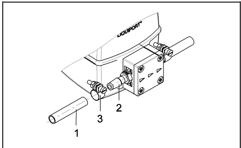
Fig. 11: Hose connector ID 8mm or ID 12mm
