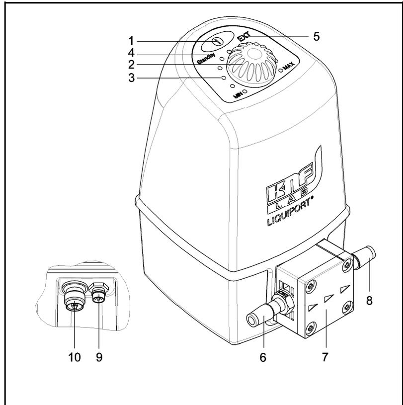
Fig. 6: Diaphragm pump
