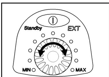
Fig. 15: Adjusting the flow rate
